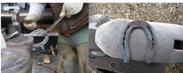
Figures 199 & 200. Gabino Fernández (2008) (Figure 199) The process is the same as for the hand horseshoes, with the proviso that in the external blade of the foot horseshoe, we emphasize the curve out of the heel, and as if we were dealing with a small American blade and (Figure 200) Mule or donkey foot horseshoe [Photographs] Accessed from http://www.farriergabino.com/
