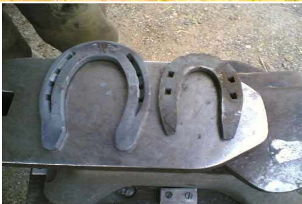
Figures 202. Gabino Fernández (2008) (Left) Donkey or mule horseshoe modified out of a horse one & (Right) Handcrafted forging donkey horseshoe [Photograph] Accessed from http://www.farriergabino.com/
