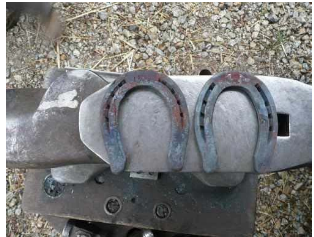
Figure 201. Gabino Fernández (2008) Donkey and mule, hand and foot horseshoes [Photograph] Accessed from http://www.farriergabino.com/
