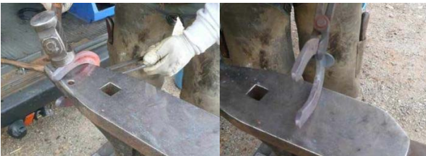
Figures 193 & 194. Gabino Fernández (2008) (Figure 193) We will hold the horseshoe at the edge of the anvil toward the second nail hole, because we want to achieve a wide toed horseshoe. We will then gently tap the horseshoe in the area behind the nail holes, to straighten the branch without damaging the grooving and stamping & (Figure 194) When straightening the branches, these remain open, so we will proceed knocking on their edge to close the horseshoe. [Fotografías] Recuperado de http://www.farriergabino.com/
