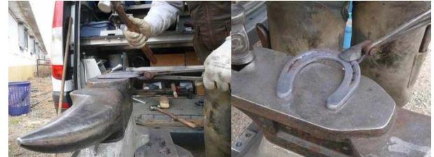
Figures 195 y 196. Gabino Fernández (2008) (Figure 195) Then we bent the faces of the horseshoe, hitting its lower face, in order to protect the grooving, (Figure 196) This is the aspect of the horseshoe once we have straightened the forks. Corns are still running inside, so you must build them in order that they turn out in its last portion, to give the horseshoe the accurate shape of the mule or ass hoof [Fotografías] Recuperado de http://www.farriergabino.com/
